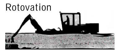
Rotovators are floating machines that use underwater rototiller-like blades to uproot aquatic plants. Rotovation is not an appropriate technique for addressing early infestations of aquatic noxious weeds.
